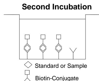
Following incubation unbound biotin-conjugated anti-mouse VEGF-A antibody is removed during a wash step. Streptavidin-HRP is added and binds to the biotin-conjugated anti-mouse VEGF-A antibody.
