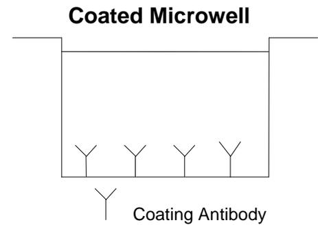
Mouse VEGF-A present in the sample or standard binds to antibodies adsorbed to the microwells.
