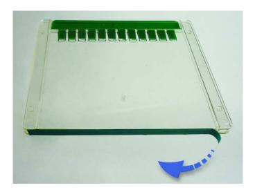
Figure 1. Peel the tape off from the bottom of the cassette
