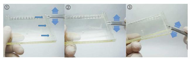
Figure 6. Open the gel cassette and remove the gel.
