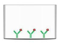
Target antigen present in standard or sample is bound by capture antibodies on the solidphase.
