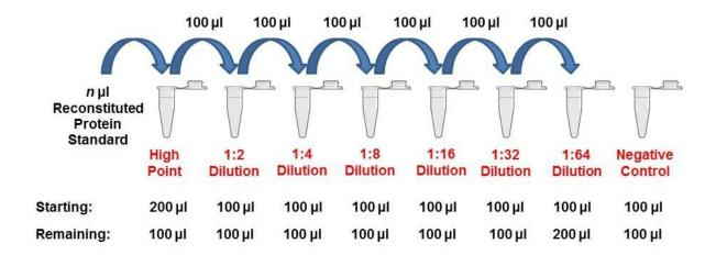
For samples of unknown protein concentrations, serial dilute the experimental sample using Sample Diluent to determine range of detection and acceptable dilutions. Shown below is a diagram illustrating a 10-fold serial dilution on a given Sample of Interest.
