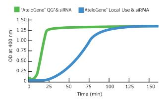
Speed of fibril formation in an "AteloGene" QG" and siRNA mixture (green line) and in an AteloGene" Local Use and siRNA mixture (blue line) at 37°C.
