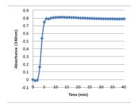
Figure 4. Polymerization of HiLyte Fluor<sup>™</sup> 647 labeled tubulin protein. Labeled tubulin protein at 5 mg/ml was resuspended in ice cold G-PEM plus 5% (v/w) glycerol. Tubulin was pipetted into a pre-warmed 96-well plate and incubated at 37°C for 40min. The increase in OD340nm over the first 10 min is indicative of microtubule polymerization.
