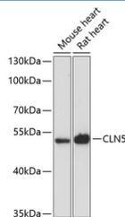
Western blot analysis of extracts of various cell lines using CLN5 Polyclonal Antibody at dilution of 1:3000.
