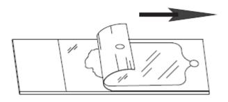
Note: HybriWells cannot be removed from coverslips.
