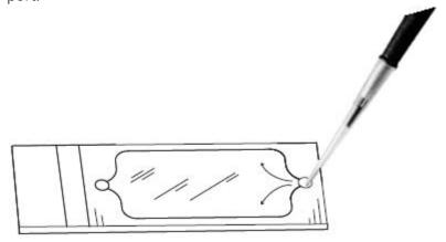
Viscous reagents may be pipetted directly onto the chamber surface of the HybriWell before the microscope slide is applied. Follow remaining steps for application and filling.
