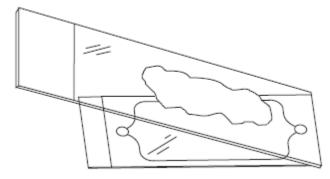
3. Ensure a secure seal by pressing the surface of the HybriWell over the adhesive area with the flat edge of the smoothing tool provided or by rubbing the HybriWell surface gently against the edge of the lab bench. Visual inspection of the adhesive area will reveal the quality of the seal.
