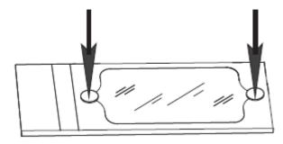
Seal tabs adhere to most wet surfaces; however, excess reagent on the HybriWell surface may be wiped away with a tissue before seal tabs are applied. Take care not to "wick" reagents from the port.
