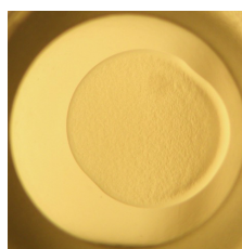
pH 9.3 Glycine Precipitate / Phase Separation
