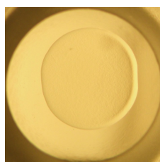
pH 8.8 Glycine Precipitate / Phase Separation
