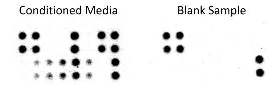
The preceding figures present typical images obtained with RayBio Dolphin Cytokine Array 1. These membranes were probed with conditioned media from a treated cell line or media blank respectively.
