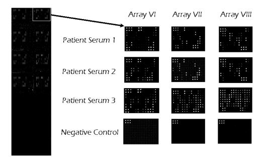
The 6 strong signals of the Positive Control spots in the upperleft corner are useful for proper orientation of the array image. If scanned using optimal scan settings, 3 distinct Positive Control signal intensities will be seen: POS1>POS2>POS3. If all of these signals are of similar intensity, try increasing or decreasing laser power and/or signal gain settings.
