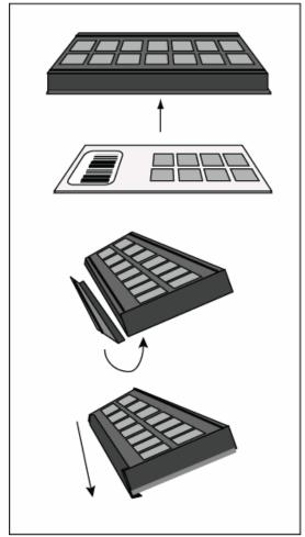
Carefully place slide at bottom of the chamber as shown. The slide will adhere somewhat to the bottom. Warning: the slide is fragile, so do not apply more than gentle force to the apparatus.
