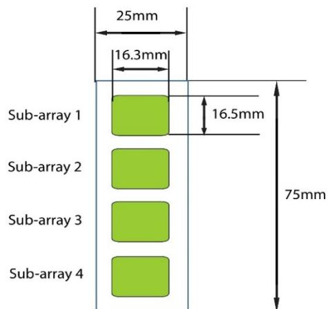
4 printed sub-arrays per glass chip
