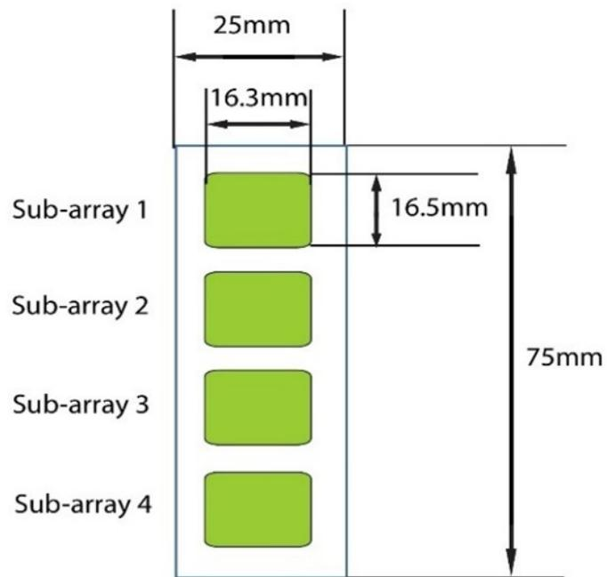
4 printed sub-arrays per glass chip
