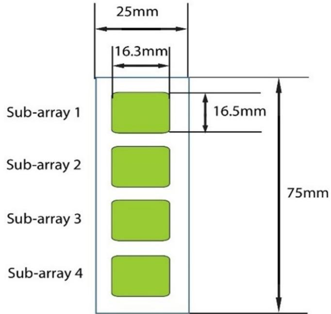
4 printed sub-arrays per glass chip
