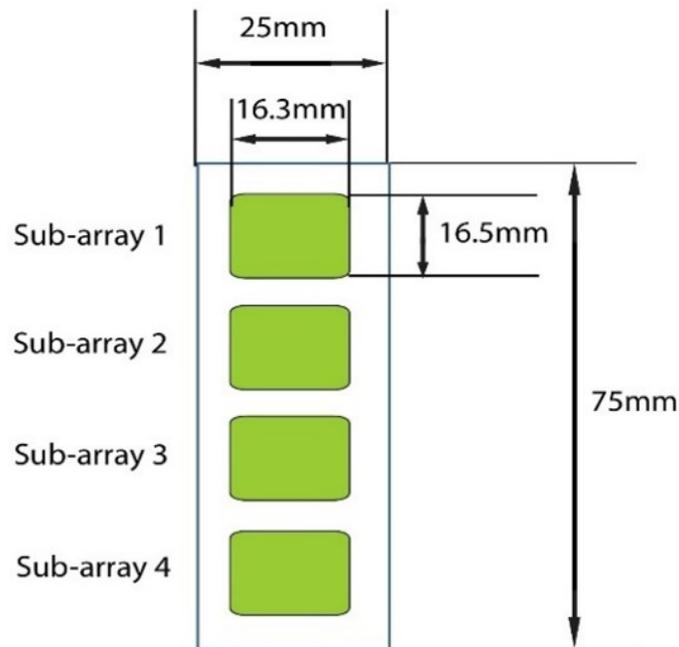
4 printed sub-arrays per glass chip
