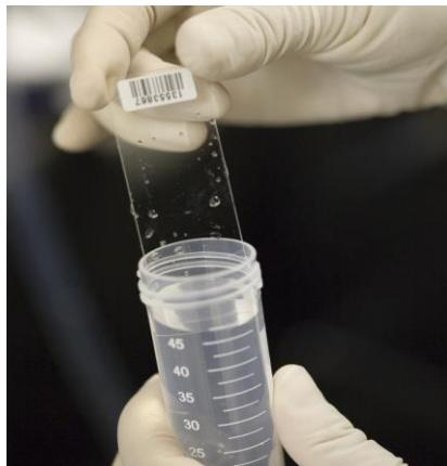
10. Wash the glass slide with 40 ml of Wash Buffer II for 5 min. Repeat one more time for a total of 2 washes.
