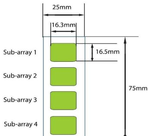
4 printed sub-arrays per glass chip
