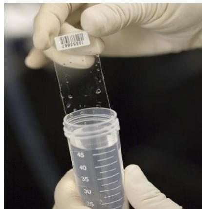
13. Wash the glass slide with 40 ml of Wash Buffer II for 5 min. Repeat one more time for a total of 2 washes.
