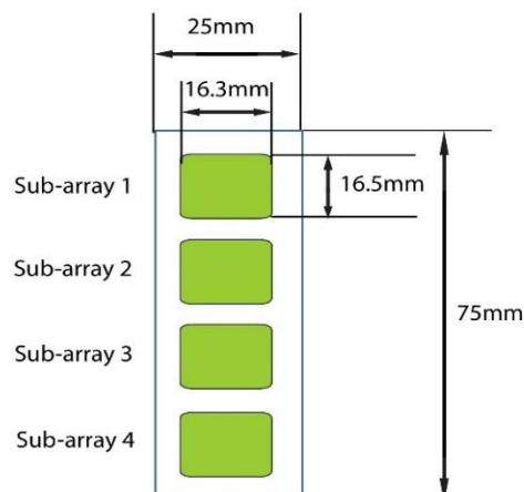
4 printed sub-arrays per glass chip
