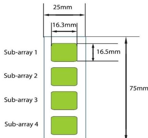
4 printed sub-arrays per glass chip
