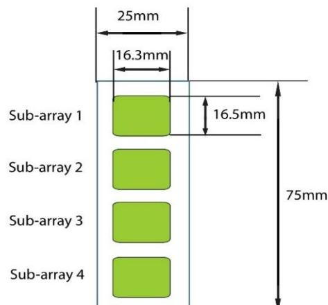
4 printed sub-arrays per glass chip
