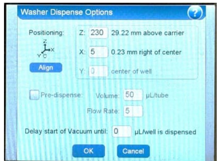
*Note: To ensure the buffer used is the 1X Wash Buffer, the Microplate Washer should be primed (250 mL) before washing the plate. Prime and one round of wash should consume 350 mL 1X Wash Buffer.*
