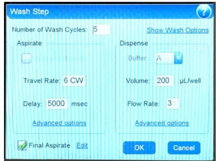
2. Wash-Aspiration: Travel Rate: 6 CW, Delay: 5 s, Alignment: X: 30, Z: 129
