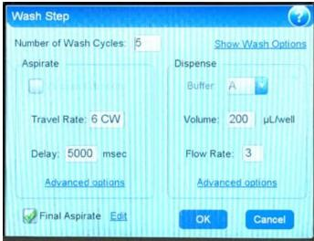
2. Wash-Aspiration: Travel Rate: 6 CW, Delay: 5 s, Alignment: X: 30, Z: 129
