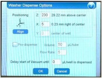
Note: To ensure the buffer used is the 1X Wash Buffer, the Microplate Washer should be primed (250 mL) before washing the plate. Prime and one round of wash should consume 350 mL 1X Wash Buffer.
