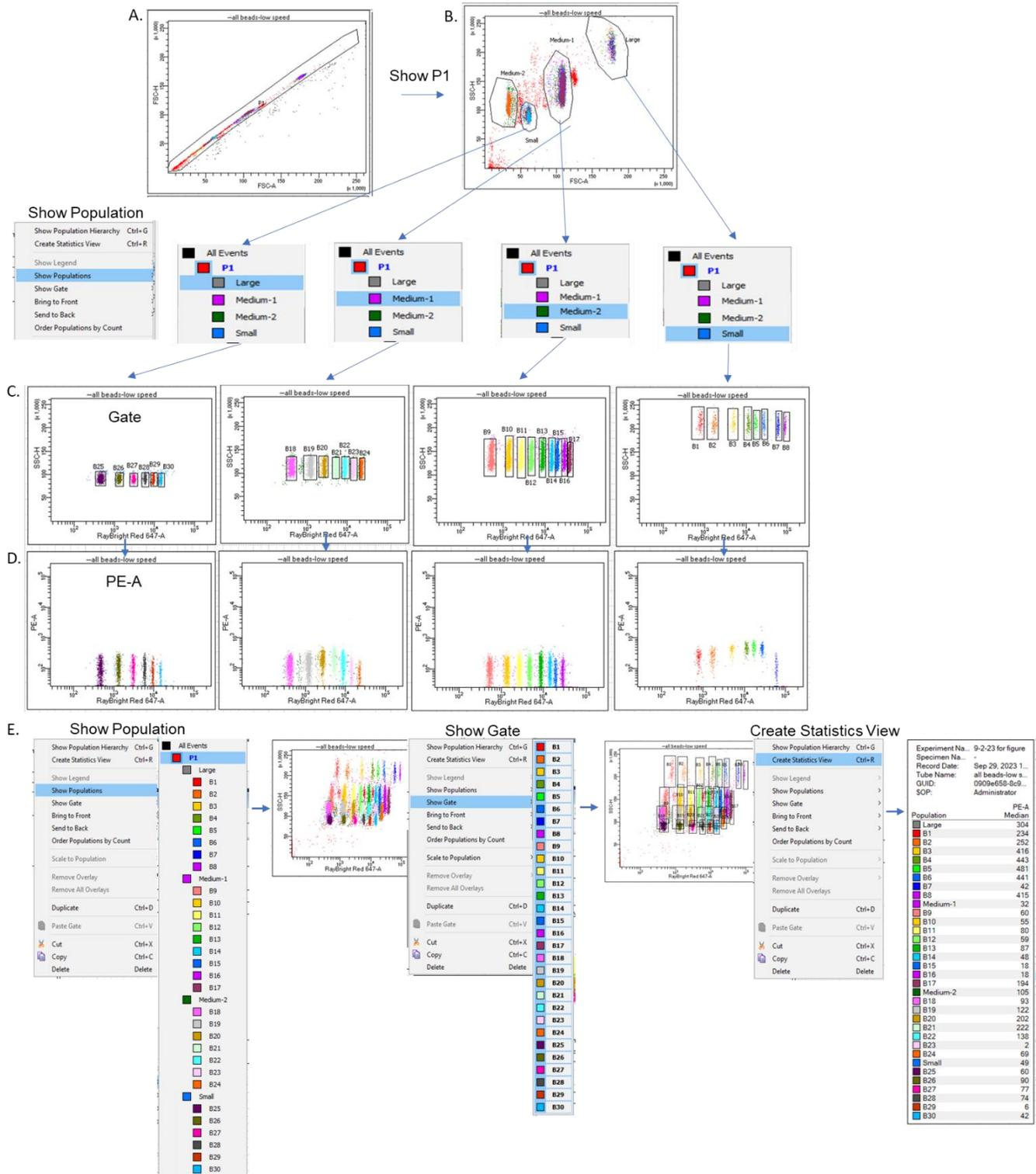
**Figure 3. Representative Images of Gated Flow Cytometry Scatter Plots Using RayPlex Arrays with small, medium-1, medium-2, and large beads. (A) Single beads are (B) separated by size, then by (C) dye concentration. (D) Beads are read based on PE-A concentration. (E) All raw PE-A Median values based on Gate of (C).**
