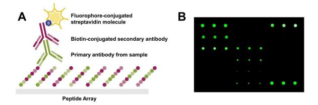
Figure 1. How peptide arrays work. A) Schematic showing that a sample primary antibody binds to its specific epitope on the peptide array. The primary antibody is detected via a biotin-streptavidin-fluorophore complex. B) A representative fluorescent image of a peptide array obtained with a compatible laser scanner. Each peptide was printed in triplicate. Green spots represent primary antibody binding to the array.
