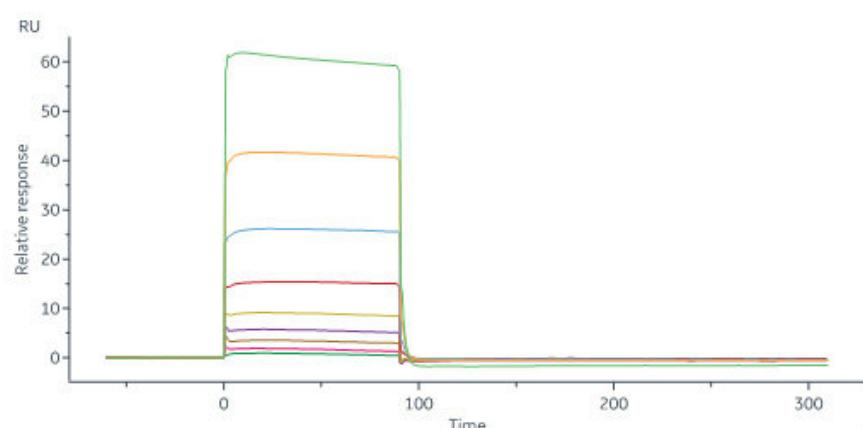
Human TIE2, Fc Tag (Cat. No. TI2-H5255) captured on Protein A Chip can bind Biotinylated Human Angiopoietin-2, His,Avitag (Cat. No. AN2-H82E7) with an affinity constant of 2.02 µM as determined in a SPR assay (Biacore 8K) (Routinely tested).
