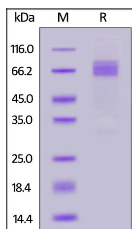
Mouse Angiopoietin-2, His Tag on SDS-PAGE under reducing (R) condition. The gel was stained with Coomassie Blue. The purity of the protein is greater than 90%.
