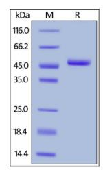
Human BAFF, Fc Tag on SDS-PAGE under reducing (R) condition. The gel was stained overnight with Coomassie Blue. The purity of the protein is greater than 95%.
