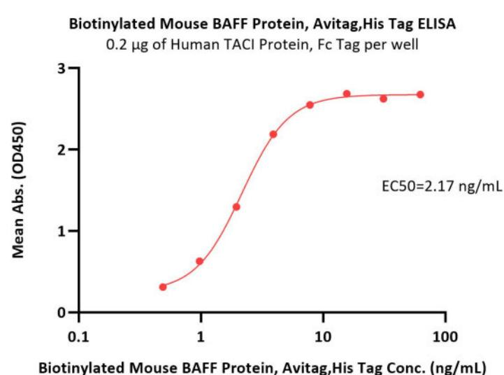
Immobilized Human TACI Protein, Fc Tag at 2 µg/mL (100 µL/well) can bind Biotinylated Mouse BAFF Protein, Avitag,His Tag (Cat. No. BAF-M82Q3) with a linear range of 0.4-4 ng/mL (Routinely tested).
