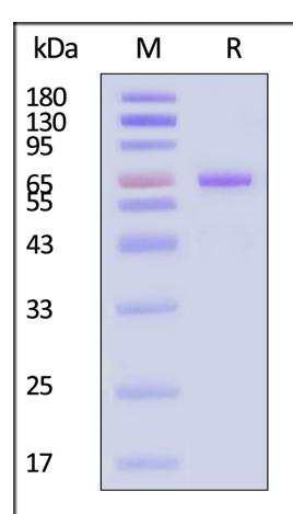
Human Cadherin-3, His Tag on SDS-PAGE under reducing (R) condition. The gel was stained with Coomassie Blue. The purity of the protein is greater than 90% (With [Star Ribbon Pre-stained Protein Marker](#)).**Bioactivity-ELISA****Discounts, Gifts,
