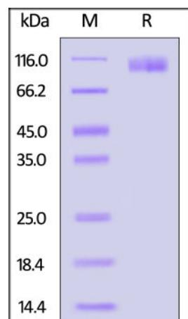
Cynomolgus CA125 Protein, His Tag on SDS-PAGE under reducing (R) condition. The gel was stained with Coomassie Blue. The purity of the protein is greater than 90%.
