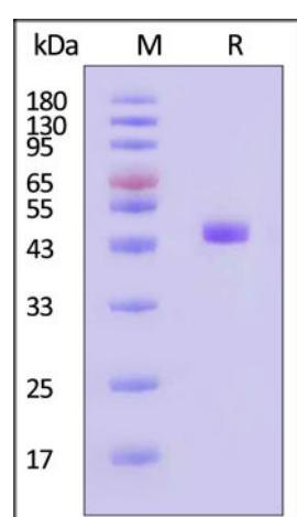
Human Cathepsin D Protein, His Tag on SDS-PAGE under reducing (R) condition. The gel was stained with Coomassie Blue. The purity of the protein is greater than 95% (With [Star Ribbon Pre-stained Protein Marker](#)).
