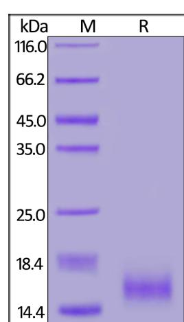
Human CD59, His Tag on SDS-PAGE under reducing (R) condition. The gel was stained with Coomassie Blue. The purity of the protein is greater than 95%.
