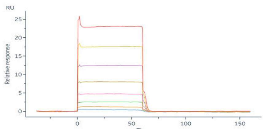
Rituximab immobilized on CM5 Chip can bind Human CD32a (H167) Protein, Strep Tag (Cat. No. CDA-H5284) with an affinity constant of 1.9  $\mu$ M as determined in a SPR assay (Biacore 8K) (Routinely tested).
