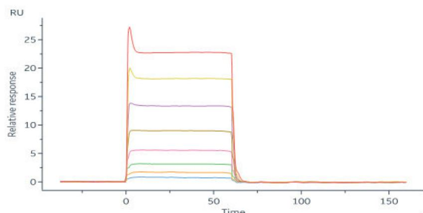
Human CD32a (H167) Protein, Strep Tag (Cat. No. CDA-H5284) immobilized on CM5 Chip can bind Rituximab with an affinity constant of 1.47  $\mu$ M as determined in a SPR assay (Biacore 8K) (QC tested).
