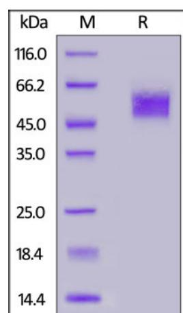
Human CD16a (V176), SUMO,His Tag on SDS-PAGE under reducing (R) condition. The gel was stained with Coomassie Blue. The purity of the protein is greater than 90%.
