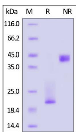
Canine CD3E & CD3D Heterodimer Protein, His Tag&Tag Free on SDS-PAGE under reducing (R) and non-reducing (NR) conditions. The gel was stained with Coomassie Blue. The purity of the protein is greater than 90%.
