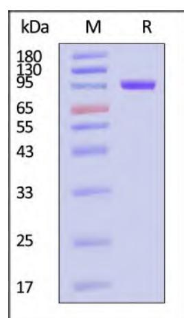
Biotinylated Human FAP Protein, His,Avitag on SDS-PAGE under reducing (R) condition. The gel was stained with Coomassie Blue. The purity of the protein is greater than 95% (With [Star Ribbon Pre-stained Protein Marker](#)).
