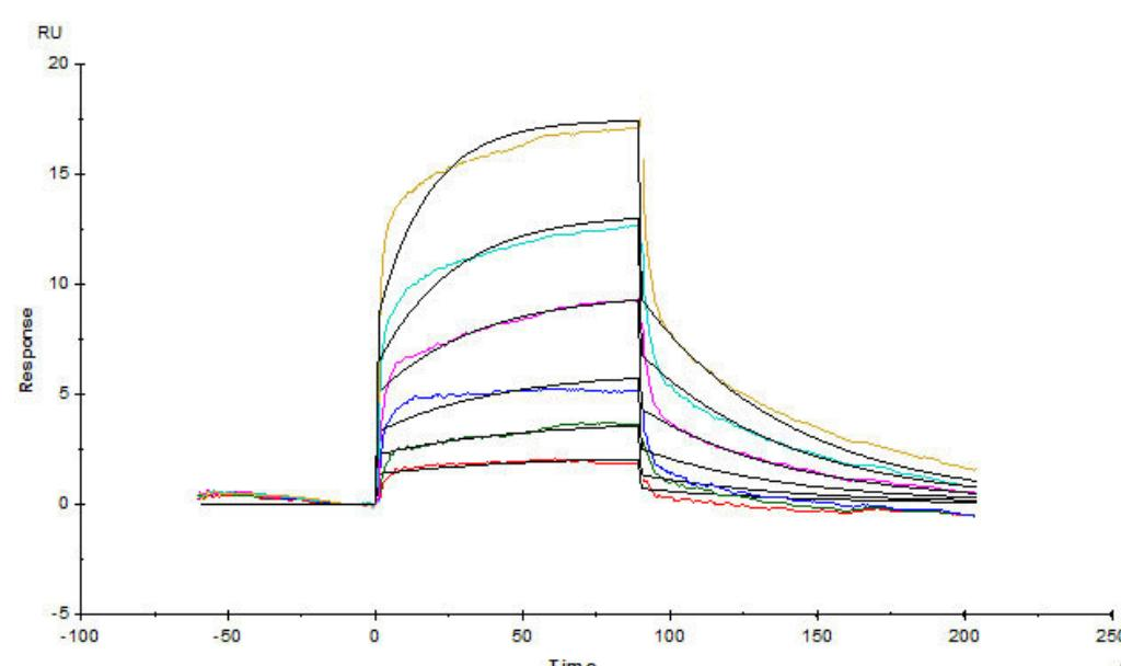
Captured Biotinylated Cynomolgus CD16, His,Avitag (Cat. No. FC6-C82E0) on Biotin CAP - Series S sensor Chip can bind MabThera® (Rituximab) with an affinity constant of 0.63  $\mu$ M as determined in a SPR assay (Biacore T200) (Routinely tested).
