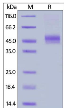
Biotinylated Cynomolgus CD64, His,Avitag on SDS-PAGE under reducing (R) condition. The gel was stained with Coomassie Blue. The purity of the protein is greater than 90%.
