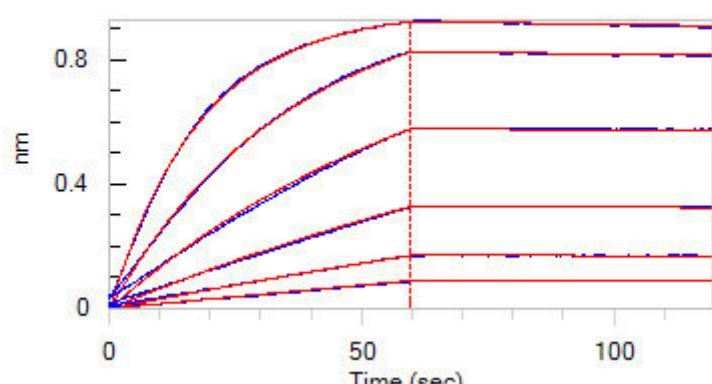
Loaded Biotinylated Cynomolgus CD64, His,Avitag (Cat. No.FCA-C82E8) on SA Biosensor, can bind Herceptin with an affinity constant of 0.326 nM as determined in BLI assay (ForteBio Octet Red96e) (QC tested).
