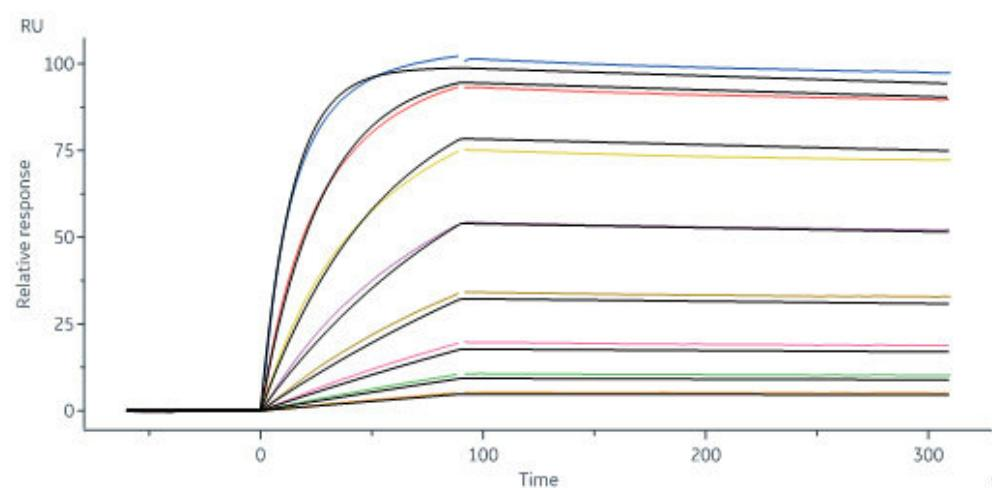
Biotinylated Cynomolgus CD64, His,Avitag (Cat. No. FCA-C82E8) captured on Biotin CAP - Series S sensor Chip can bind Herceptin with an affinity constant of 1.50 nM as determined in a SPR assay (Biacore 8K) (Routinely tested).
