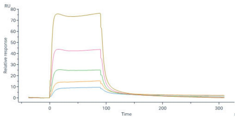
Human FGF R4, Fc Tag (Cat. No. FG4-H5253) immobilized on CM5 Chip can bind Human FGF-4 Protein, His Tag (Cat. No. FG4-H51H3) with an affinity constant of 1.48  $\mu$ M as determined in a SPR assay (Biacore 8K) (QC tested).
