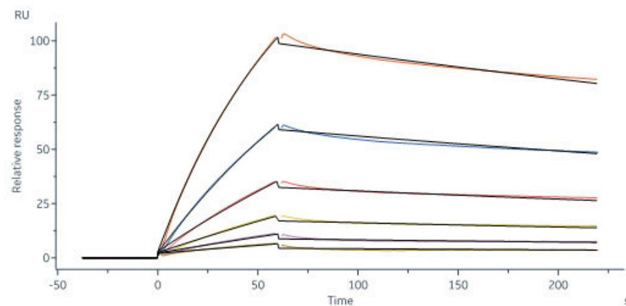
Biotinylated Human FGF basic, Avitag,His Tag (Cat. No. FGC-H81E3) immobilized on SA Chip can bind Human FGF R1, His Tag (Cat. No. FG1-H5223) with an affinity constant of 96.3 nM as determined in a SPR assay (Biacore 8K) (Routinely tested).
