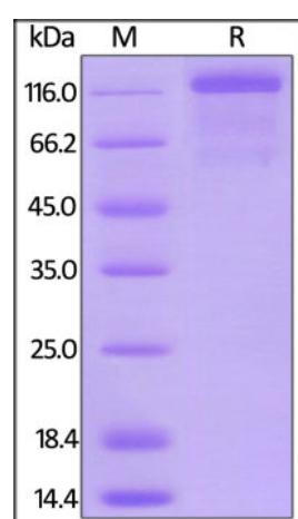
Mouse VEGF R3 Protein, Mouse IgG2a Fc Tag on SDS-PAGE under reducing (R) condition. The gel was stained with Coomassie Blue. The purity of the protein is greater than 95%.
