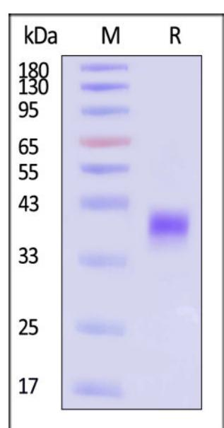
FITC-Labeled Human FOLR1, His Tag on SDS-PAGE under reducing (R) condition. The gel was stained with Coomassie Blue. The purity of the protein is greater than 95% (With [Star Ribbon Pre-stained Protein Marker](#)).
