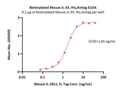
Immobilized Biotinylated Mouse IL-33, His,Avitag (Cat. No. IL3-M82Q7) at 1  $\mu$ g/mL (100  $\mu$ L/well) on streptavidin (Cat. No. STN-N5116) precoated (0.5  $\mu$ g/well) plate can bind Mouse IL-1RL1, Fc Tag (Cat. No. IL1-M5259) with a linear range of 0.05-5 ng/mL (QC tested).
