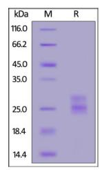
Biotinylated Mouse IL-33, His, Avitag on SDS-PAGE under reducing (R) condition. The gel was stained with Coomassie Blue. The purity of the protein is greater than 90%.
