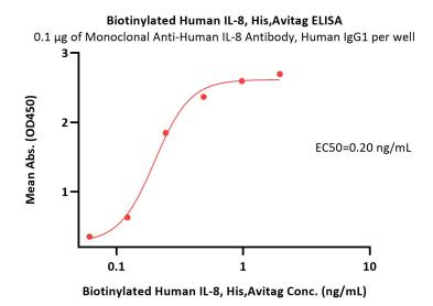
Immobilized Monoclonal Anti-Human IL-8 Antibody, Human IgG1 at 1  $\mu g/mL$  (100  $\mu L/well)$  can bind Biotinylated Human IL-8, His,Avitag (Cat. No. IL8-H82H3) with a linear range of 0.06-0.24 ng/mL (Routinely tested).
