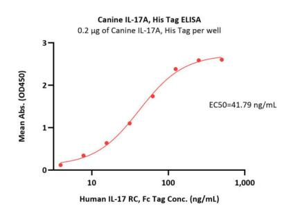
Immobilized Canine IL-17A, His Tag (Cat. No. ILA-C52H7) at 2  $\mu$ g/mL (100  $\mu$ L/well) can bind Human IL-17 RC, Fc Tag with a linear range of 4-63 ng/mL (Routinely tested).
