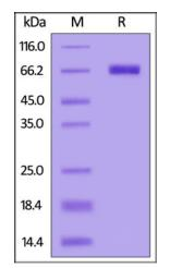
Human KIR2DL3, Fc Tag on SDS-PAGE under reducing (R) condition. The gel was stained with Coomassie Blue. The purity of the protein is greater than 95%.
