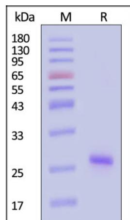
Human KRAS Protein, His Tag on SDS-PAGE under reducing (R) condition. The gel was stained with Coomassie Blue. The purity of the protein is greater than 95% (With [Star Ribbon Pre-stained Protein Marker](#)).
