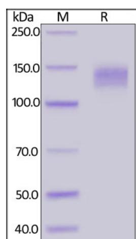
Rabbit LDL R, Fc Tag on SDS-PAGE under reducing (R) condition. The gel was stained with Coomassie Blue. The purity of the protein is greater than 90%.
