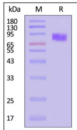
Human LIV-1, Fc Tag on SDS-PAGE under reducing (R) condition. The gel was stained with Coomassie Blue. The purity of the protein is greater than 95% (With [Star Ribbon Pre-stained Protein Marker](#)).
